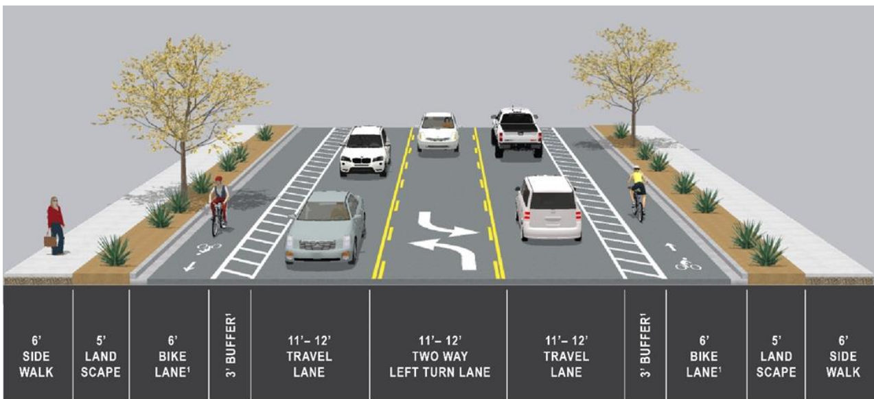
Figure 5 Three-Lane Collector Proposed Cross-Section
