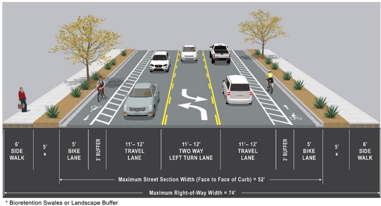
Figure 5 Three-Lane Minor Arterial Cross-Section
